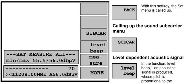
received signal level. With it, it is possible to optimally align the receiving antenna to a transmitter.
